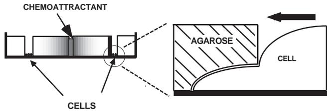
**Fig. 1.** Under-agarose chemotactic assay. Three parallel troughs are cut into the agarose. The center trough is filled with folate and cells are placed in the peripheral troughs. Cells then migrate towards the folate, deforming the agarose upwards while simultaneously flattening themselves. Arrow indicates direction of cell movement.
