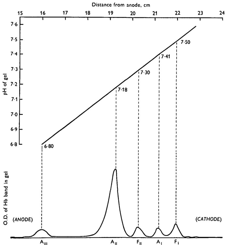
Fig. 2. Optical density scan (420 nm) of hamster haemoglobins (at day of birth) separated by isoelectric focusing in polyacrylamide gel. The haemoglobins migrate to positions in the linear portion of the pH gradient. Haemoglobin peaks are matched here with their isoelectric points measured directly in the gel.
